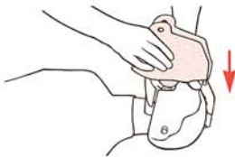
Turn manikin face inside out and push face coupling into airway valve.
